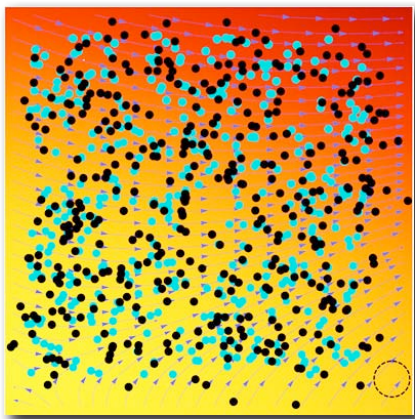
Figure 8. Arrows visualize flow inferred from a set of identical particles in two consecutive images. Black indicates the initial position of the particles, and blue indicates the final position. The circle in the right corner shows the strength of diffusion.
